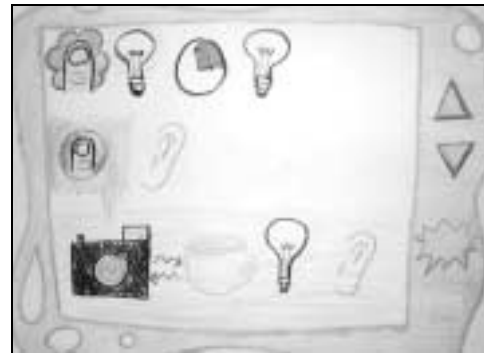
Figure 5: Some early visual programming ideas. The top line means "press the flower and the light stays on for 15 seconds." The third line means "when the camera and the cup are near each other, the light comes on and the ear will listen."
