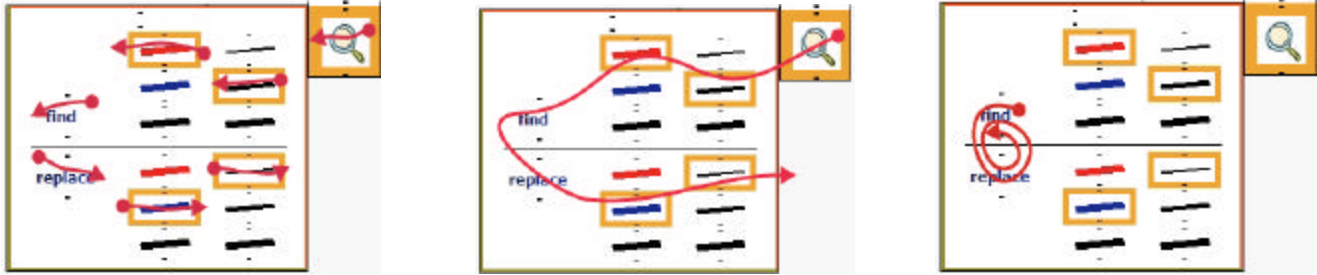
Figure 7 (left) Using single strokes on the find and replace panel. (middle) Combining the single strokes into one stroke. (right) Repeated find-and-replace operations using a continuous stroke.
